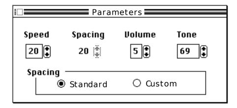
The controls operate the same as the controls in the Alarm Clock desk Accessory. Speed sets the Morse code sending speed over the range of 4 to 30 words per minute. Volume adjusts the volume from 1 to 7 (1 to 7 have the same meaning as they do in the control panel).
