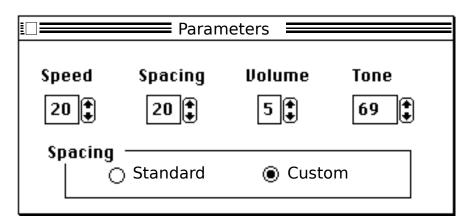
Custom spacing allows you to send individual characters at higher speeds and space them at a lower speed. In the custom spacing mode the speed control sets the character speed and the spacing control sets the space between characters. This allows you to get used to the sound of characters at high speed while still being able to copy at a slower speed.
